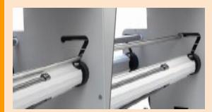
✓ Clear static device to remove static during laminating
